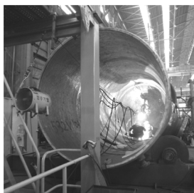
(a) Tunnel type of limited space
