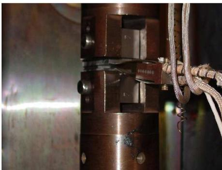
Fig. 11 Appearance of fracture toughness test
