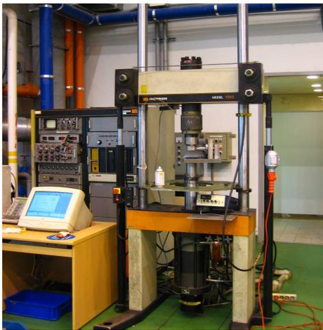
Fig. 10 Experimental setup for fracture toughness test
