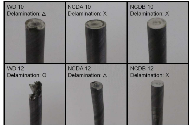
Fig. 2 Observations of the fracture surfaces of twisted wires processed by the WD, NCDA, and NCDB, respectively
