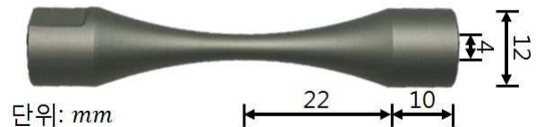
Fig. 3 Al6061 specimen for UFT at 20 kHz
