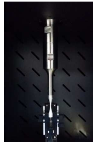
Fig. 4 Ultrasonic fatigue tester(UFT-20X, MediSource-Plus corp.)
