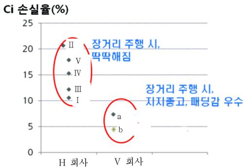
Fig. 6 Loss ratio of Ci for different seats
