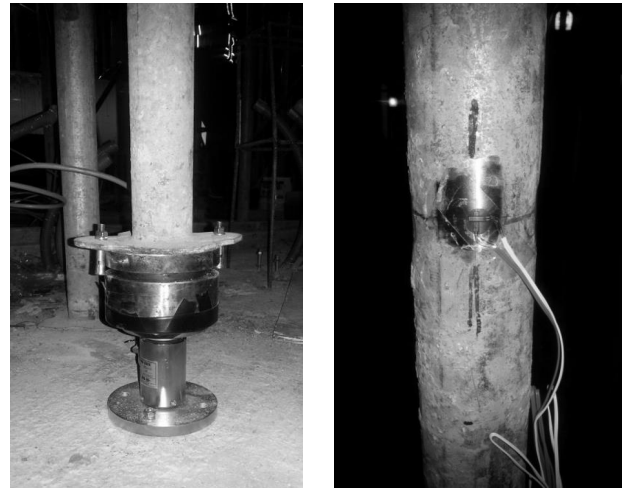
(a) Load cell at the base of (b) Strain gage at a shore a shore
