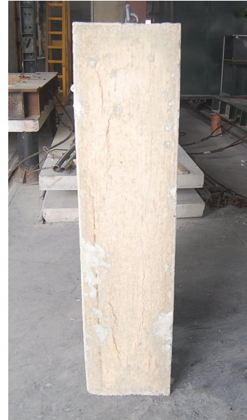
Fig. 5 Appearance observation of the specimen after fire test
