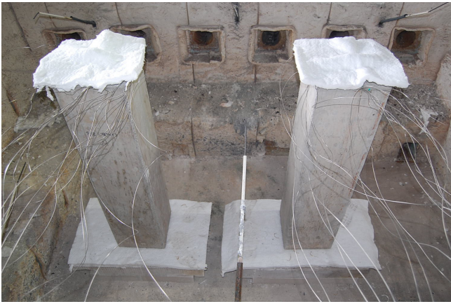
Fig. 3 Fire test set-up of RC columns
