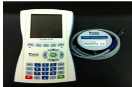
Fig. 2. Thermal conductivity device (ISOMET 2114)
