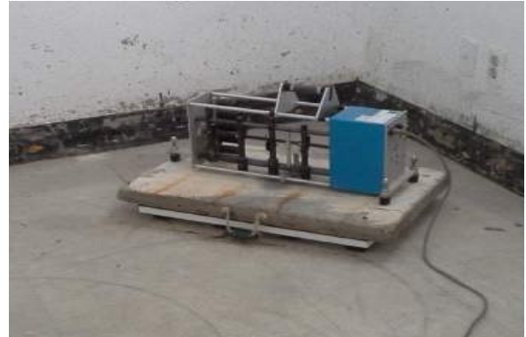
(a) Lightweight impact test (equipment : tapping machine)
