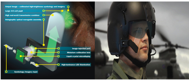
FIG. 7. Key functional component of Q-sight 100 display of BAE system and experimental flight prototype.
