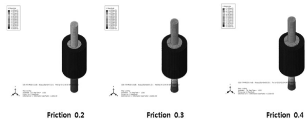
Fig. 5. Deformation of anchor with respect to friction coefficient
