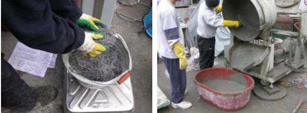
(b) Steel fiber of indent shape (c) Cement mortar mixing
