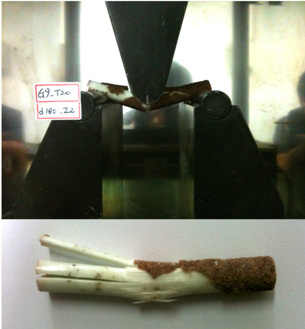
Photo 4 Interlaminar shear strength test
