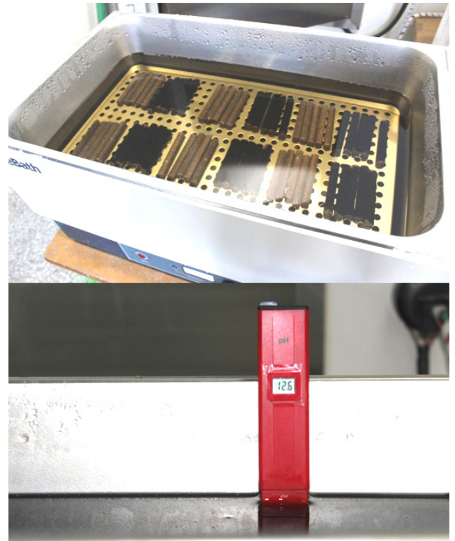
Photo 3 Conditioning in alkaline solution
