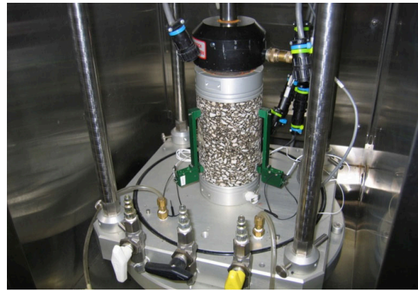
Fig. 3 Dynamic Modulus Test Set-Up
