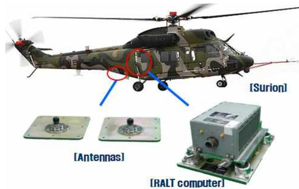
Fig. 1. RADAR altimeter set for Surion
