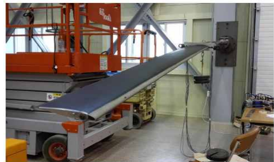
Fig. 15. Reinforced BO-105 Blade Flap Stiffness Measurement Test
