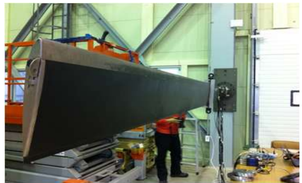
Fig. 11. Lag Stiffness Measurement Test
