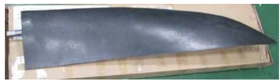
Fig. 14. Manufactured Composite Blade
