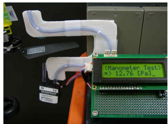
Fig. 22. Experimental Environment 2 (Differential Pressure measurement)
