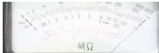
Figure 14: High speed coupling insulation resistance test and result
