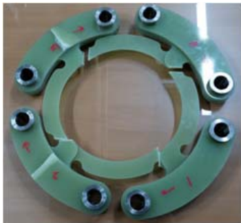
Figure 13: Fractured disc pack at 60kNm torque
