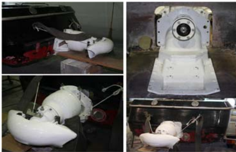
(b) Installation of water jet
