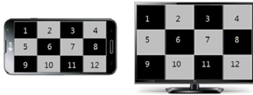
Figure 5: Position mapping of touch button between Smart TV and Smart phone.
