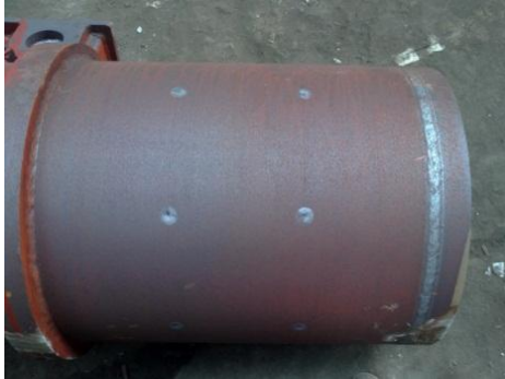
Fig. 4. The novel cooling water jacket with key hold caulks weld spots
