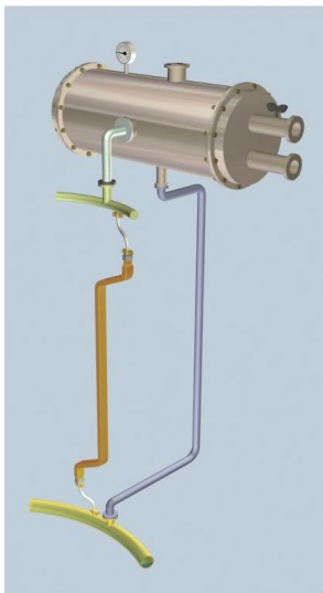
Fig. 1. Schematic diagram of evaporative cooling system of a hydro-generator
