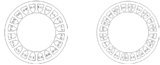
(a) GFSCW motor (b) MFSCW motor Fig. 1. Stator layouts of 20/22 five-phase motors
