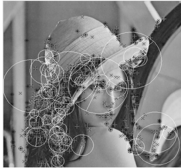
Fig. 5. Results of keypoint detection. For Lena, PSNR=43.02dB. Size of block ( 3 \times 3 ) on DoG space
