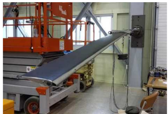
Fig. 12 Flap stiffness measurement of BO-105 blade
