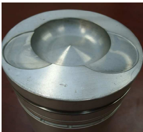
Fig. 2 A newly fabricated piston with the compression ratio of 22
