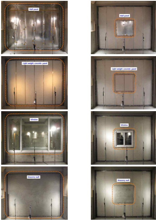
Fig. 4. Installed Test specimen of Test Room(Left : Full size, Right : Small size)
