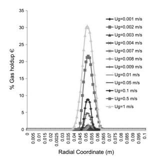
**Figure 3.** Radial distribution of gas holdup. Values measured at a height of 0.5 m from the gas distributor.
