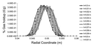
Figure 6. Radial distribution of gas holdup at varying heights.
