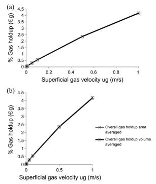
**Figure 2.** (a) Cross sectional area averaged and column volume average gas holdup as a function of low superficial gas velocity. (b) Cross sectional area averaged and column volume average gas holdup as a function of high superficial gas velocity.
