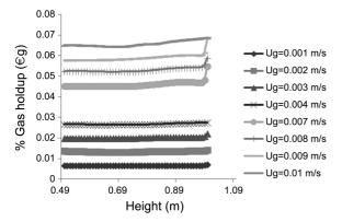
**Figure 4.** Gas Holdup Distribution along Column Height, values measured from a height of 0.5 m from gas distributer (For lower gas velocities).
