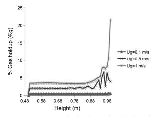
**Figure 5.** Gas Holdup Distribution along Column Height, values measured from a height of 0.5 m from gas distributer (For higher gas velocities).
