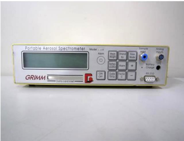
Fig. 2 Portable aerosol spectrometer
