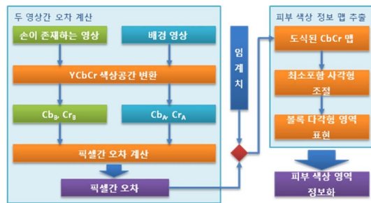
Fig. 3 Procedure for constructing a skin color map
