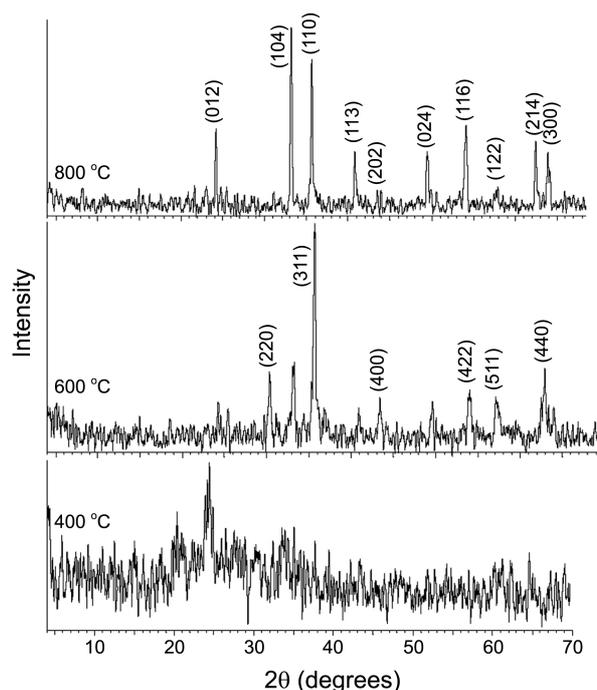
**Figure 2.** XRD patterns of gelatin-Fe<sub>3</sub>O<sub>4</sub> nanocomposite at 400 °C,  $\gamma$ -Fe<sub>2</sub>O<sub>3</sub> nanoparticles at 600 °C.
