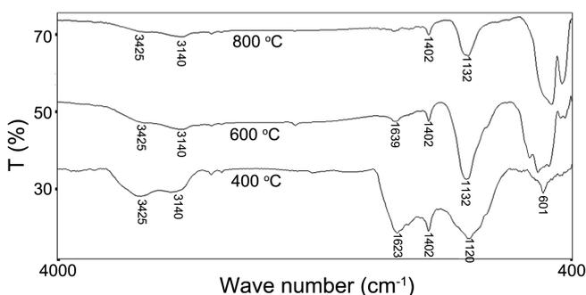
**Figure 4.** FT-IR spectra of gelatin- $\text{Fe}_3\text{O}_4$  nanocomposite at 400 °C,  $\gamma$ - $\text{Fe}_2\text{O}_3$  nanoparticles at 600 °C and  $\alpha$ - $\text{Fe}_2\text{O}_3$  nanoparticles at 800 °C.
