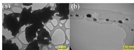
**Figure 6.** TEM images of synthesized materials (a) without any gelatin (b) using 1.0 g gelatin.
