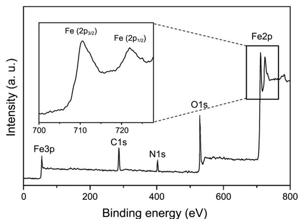
**Figure 1.** Survey scan of gelatin-Fe<sub>3</sub>O<sub>4</sub> composite and its high-resolution XPS spectrum of Fe2p.
