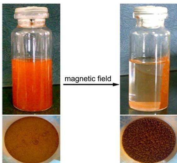
**Figure 3.** The produced maghemite nanoparticles dispersed in ethanol at absence and present of magnetic field.
