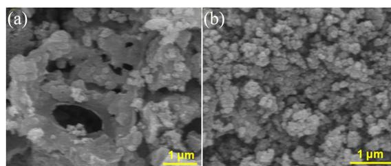
**Figure 5.** SEM images of (a) gelatin- $\text{Fe}_3\text{O}_4$  nanocomposite after 1 h curing at 500 °C and (b) synthesized  $\gamma$ - $\text{Fe}_2\text{O}_3$  nanoparticles after 1 h curing at 600 °C (complete decomposition of gelatin).
