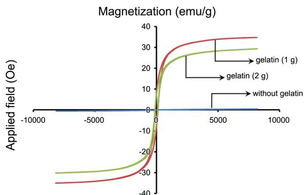
**Figure 7.** Effect of gelatin amounts on VSM hysteresis loop of synthesized materials.
