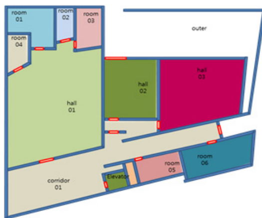
Figure 14. 2D Example of Volume-based Modeling for Building A
