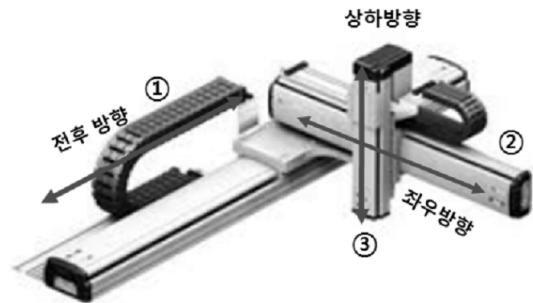
Fig. 8. Rectangular coordinates robot for tripple-degree of freedom.
