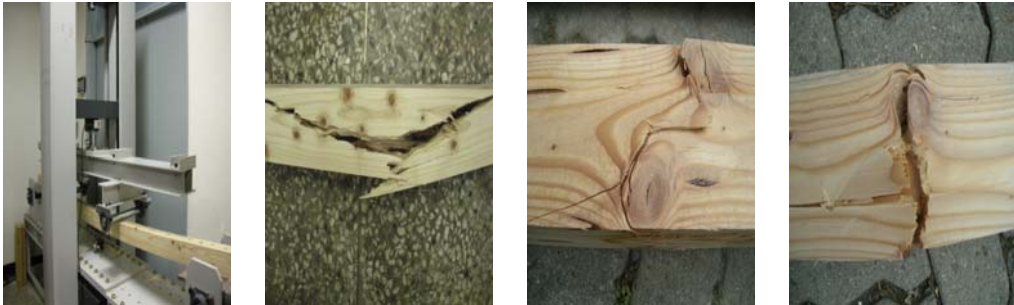
Fig. 4. failure mode of small diameter lumber.
