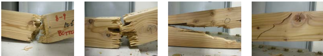
Fig. 5. failure mode of finger joint small diameter lumber.
