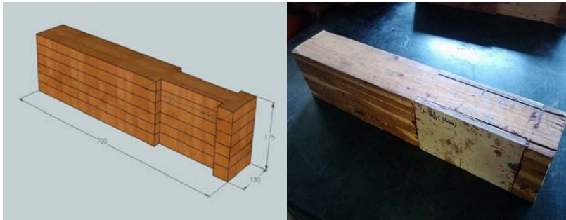
Fig. 5. Shape of reinforced beam.
