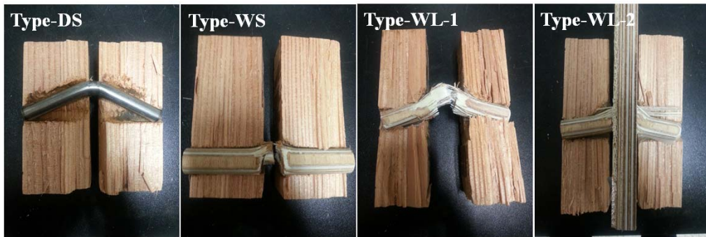
Fig. 8. Failure modes of tensile type shear strength test.
