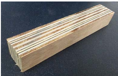
Fig. 2. Shape of rectangular GFRP reinforced laminated wooden pin.
