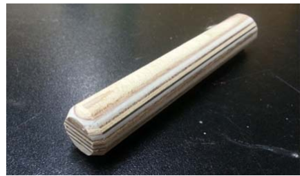
Fig. 3. Shape of circular GFRP reinforced laminated wooden pin.
