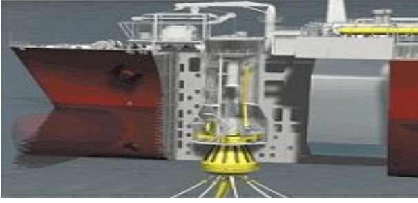
Fig. 1. General arrangement of a LNG-RV attached the STL.
