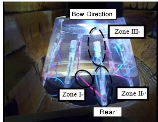
Fig. 12. Flow patterns of the inner part at the opening condition detached the STL from a vessel (Experiment).
