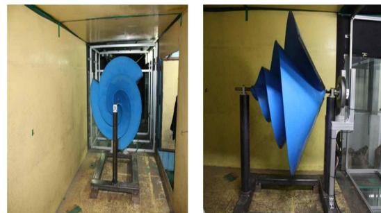
Fig. 1 The manufactured spiral blade rotor in wind tunnel
