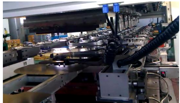
Fig.21 Press line of semi-progressive and transfer die
