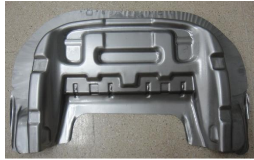
Fig.15 Drawing process of seat cushion panel
