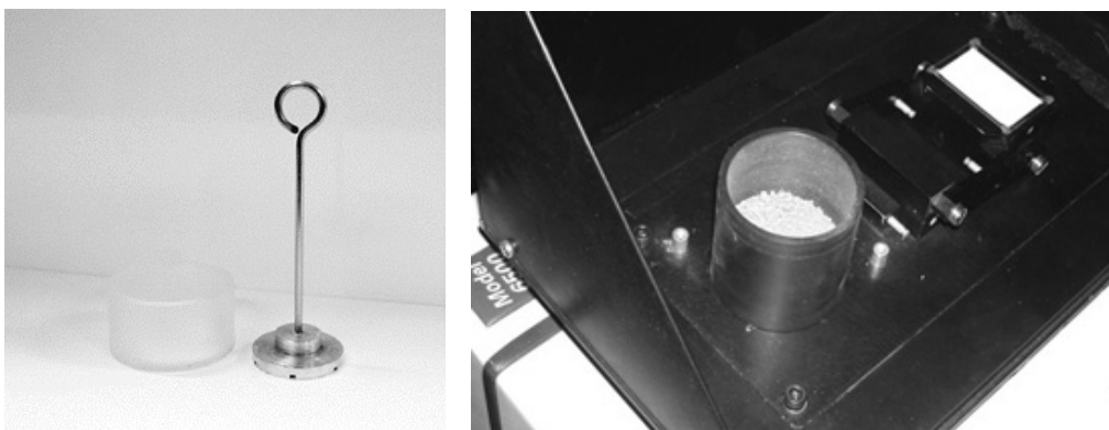
Fig. 1. Sample cell, reflectance plate (left) and horizontal type spectrophotometer (right) for reflectance spectra measurements.
