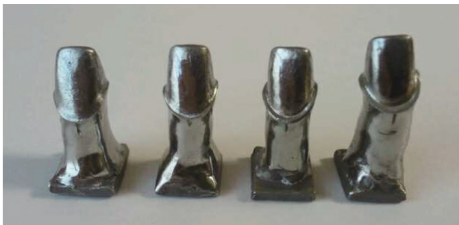
Fig. 1. Four master models used in this study (From the left side, chamfer, heavy chamfer, shoulder with bevel, and shoulder).
