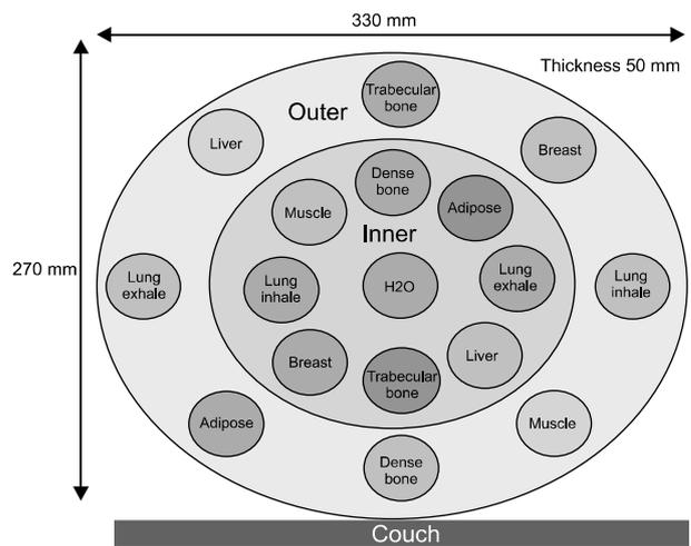
**Fig. 1.** CIRS062 phantom and Inserts position; CIRS062 phantom consists of inner (head) and outer (lung) parts. Eight different tissue equivalent inserts pairs were arranged symmetrically around the phantom center at the inner and outer region of the phantom.
