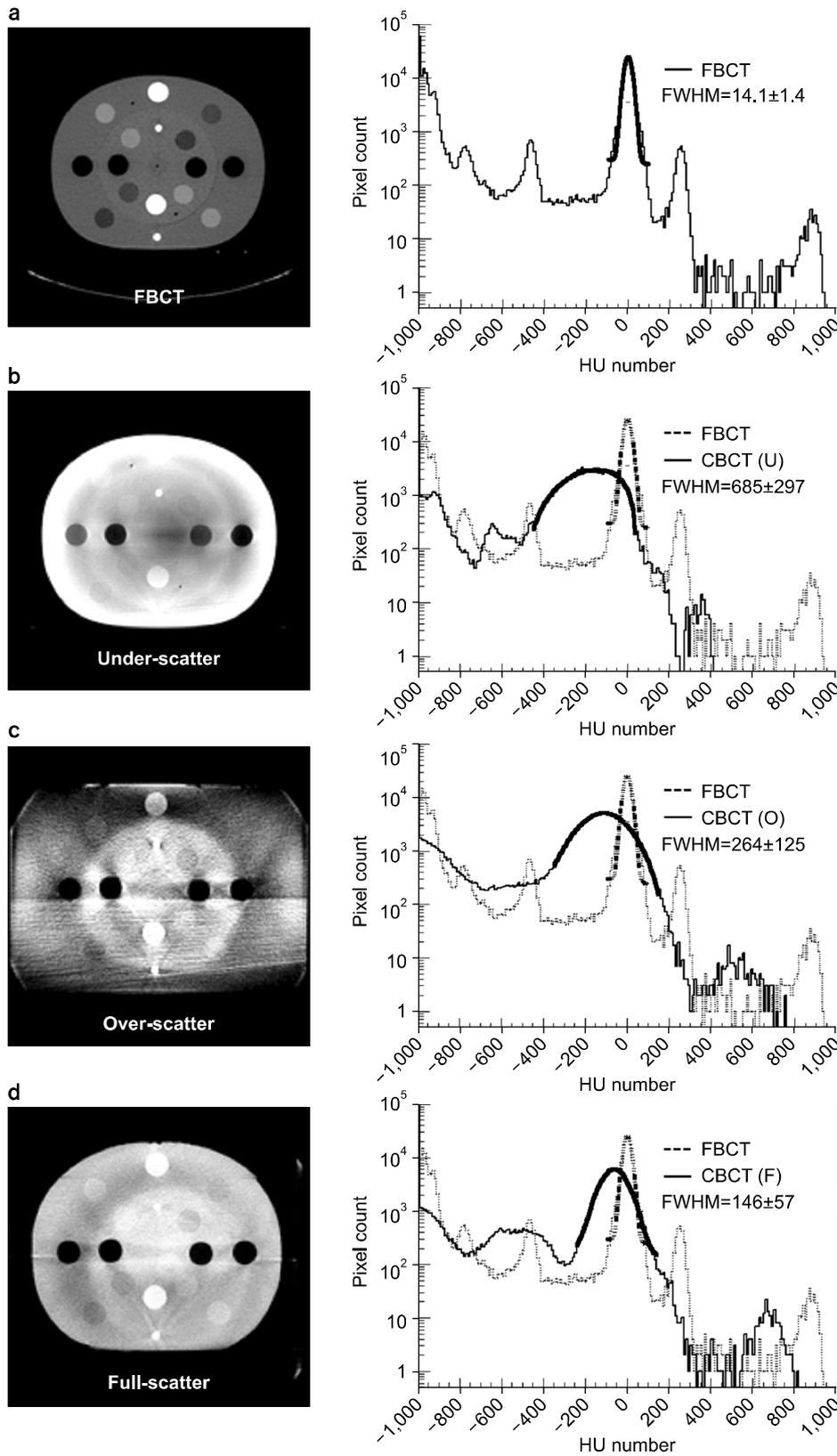
**Fig. 3.** HU histograms of the FBCT and CBCT images with various scatter conditions. (a) FBCT image and HU histogram, (b) CBCT image and histogram with “Under-scatter” condition. (c) CBCT image and histogram with “Over-scatter” condition. (d) CBCT image and histogram with “Full-scatter” condition. The main peak on each histogram represents the histogram of the water equivalent material that composes the main body of the phantom.
