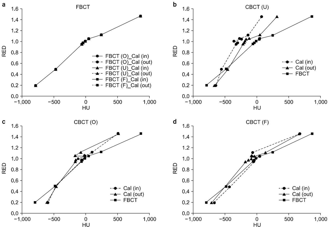
**Fig. 4.** Comparison of FBCT and CBCT HU-ED calibration curves and HU differences of the same ED insert-pairs between their locations (inner and outer parts of phantom). (a) FBCT HU-ED calibration curve with three scatter condition. (b) CBCT HU-ED calibration curve with "Under-scatter" condition. (c) CBCT HU-ED calibration curve with "Over-scatter" condition. (d) CBCT HU-ED calibration curve with "Full-scatter" condition.
