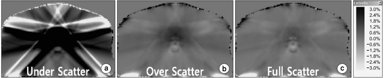
Fig. 5. Percentage dose difference map of different HU-ED calibration based CBCT dose distributions for prostate patient 1. (a) "Under-scatter" calibration curve. (b) "Over-scatter" calibration curve. (c) "Full-scatter" calibration curve.
