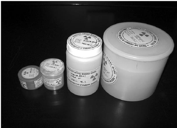
Fig. 2. The photography of various CRMs for the efficiency measurement of various measuring containers and the detection system.
