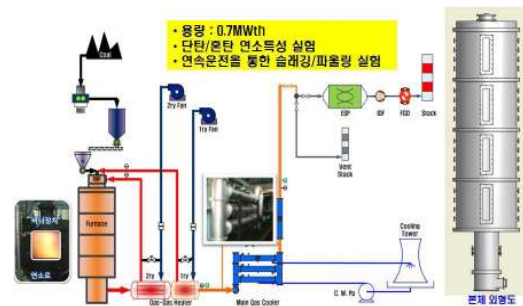
Fig. 1. Schematic Diagram of 0.7MWth Coal-fired Pilot
