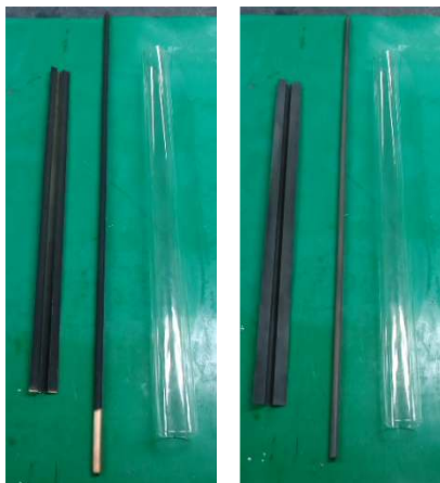
(a) Black chrome plating (b) Copper coating Fig. 1. Surface treatment of absorber plate and heat pipe.
