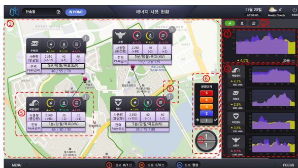
Figure 3 Graphic User Interface of urban unit monitoring - ① Location Info. ② Type of energy monitoring ③ Use of Urban energy ④ Each use of building ⑤ State of energy use ⑥ Operation level's control ⑦ Level of operation
