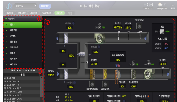
Figure 4 Graphic User Interface of system unit monitoring - ① Type of system monitoring ② List of below system ③ Monitoring field
