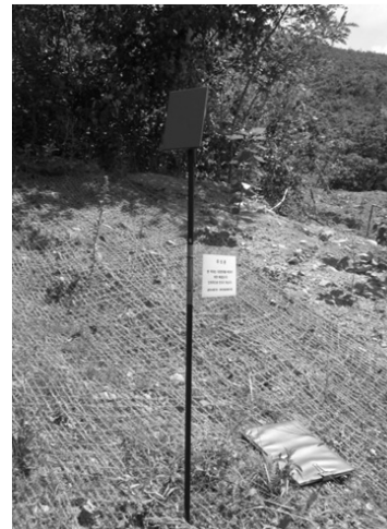
(b) Target attached to the top of steel pole
