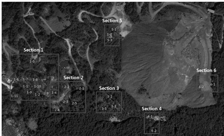
Fig. 4. Location of measurement point to measure the ground displacement
