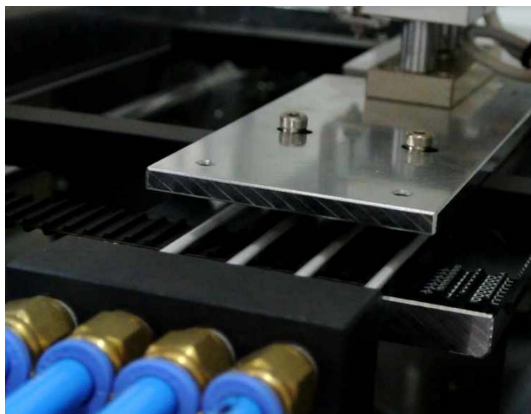
Fig. 3. Apparatus for CCFL tube transfer, mercury/fluorescence compound separation.
