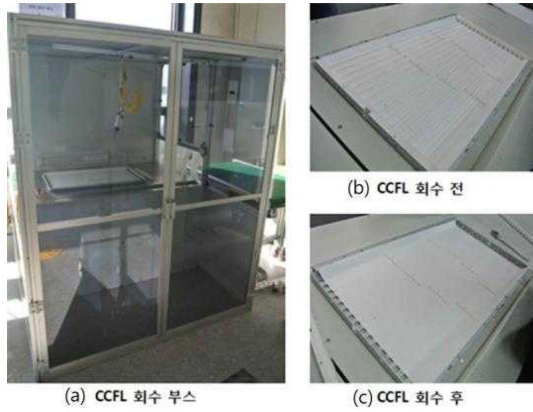
Fig. 8. (a) Booth for CCFL separation, (b) Array of CCFLs in the mold frame; (c) Mold frame after separation of CCFLs.
