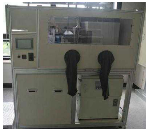
Fig. 1. CCFL decontamination system.
