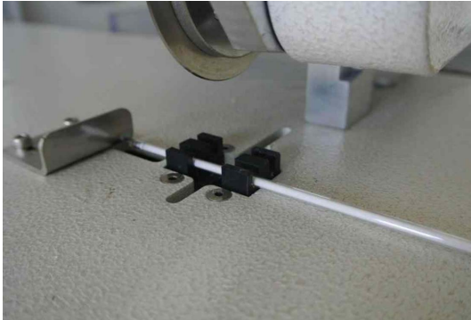
Fig. 2. Cutting apparatus and cutting operation in the CCFL decontamination system of Fig. 1.
