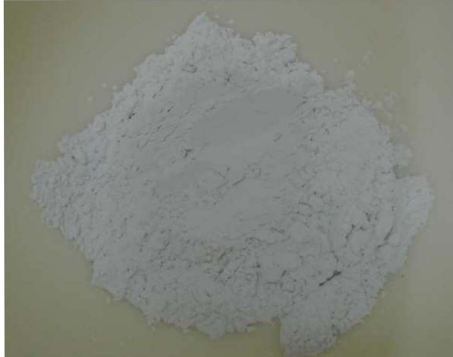
Fig. 10. Recovered powders of mercury/fluorescent compound.
