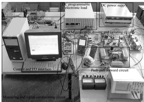
Fig. 15. Experimental setup of PV simulator.
